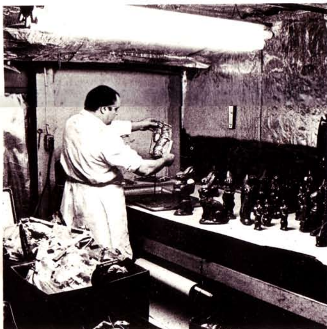
Chocolate bunnies are made by coating inside of molds with melted chocolate, then pouring off excess.
